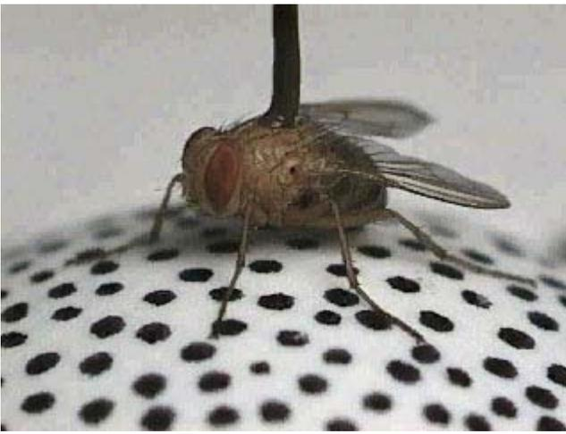
**By using a free-floating ping-pong ball as a "fly treadmill," scientists were able to measure precise changes in the fly's direction of motion. Dots on the ball enabled tracking by computer. [A quicktime movie of the fly in action](#) (3.5MB) is available. Broadcast-quality digital video is available to the media.**
